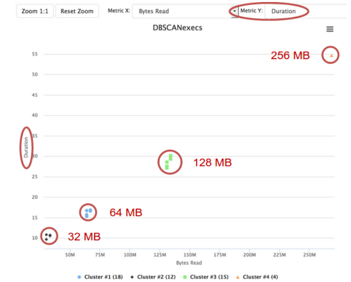
Fig. 8. Example of the DBSCAN-EXECS displaying the duration and bytes read for k-means benchmark executions, highlighting the detected block sizes
